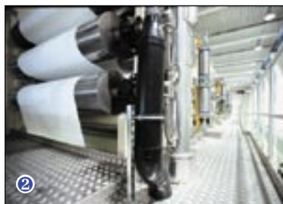
In Weissenborn, Germany, Felix Schoeller operates a unique integrated photo paper production facility. The actual paper production ① is supplemented by high-speed extruders ② for the double-sided PE coating. After converting ③, cutting and packaging, the highly efficient logistics center ensures punctual delivery of the materials – anywhere in the world ④.
